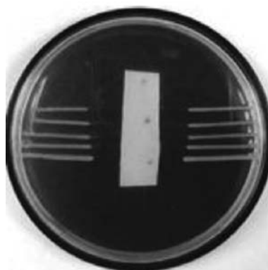
Figure 5. Left photo: Petri dish showing effectiveness of biocide component after more than four years of burial in the Everglades with 100 percent kill rate. Right photo: Flasks showing effectiveness of inhibitor with three ductile iron (DI) samples in 5 percent salt solution after five years. The flask on the right is bare DI, the flask in the middle is bare DI wrapped with conventional polyethylene encasement, and the flask on the left is bare DI wrapped in enhanced (with biocide and inhibitor) polyethylene film.
