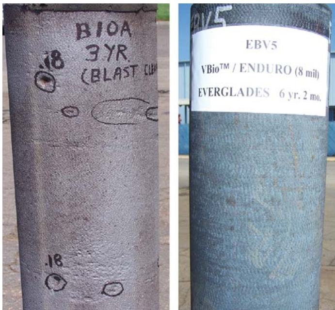
Figure 6. Left: Bare DI pipe after three years burial with corrosion pits up to 0.18 in. Right: Bare DI pipe with polyethylene encasement containing biocide and corrosion inhibitor after six years burial in the Everglades with zero pitting.
