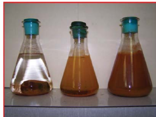
Figure 5. Left photo: Petri dish showing effectiveness of biocide component after more than four years of burial in the Everglades with 100 percent kill rate. Right photo: Flasks showing effectiveness of inhibitor with three ductile iron (DI) samples in 5 percent salt solution after five years. The flask on the right is bare DI, the flask in the middle is bare DI wrapped with conventional polyethylene encasement, and the flask on the left is bare DI wrapped in enhanced (with biocide and inhibitor) polyethylene film.
